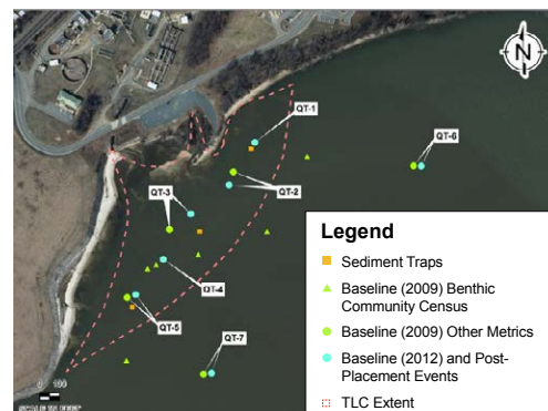
Figure 3. Site 99 TLC Extent at Quantico Embayment at Quantico MCB showing Sediment Trap Placement and Baseline Sampling Locations (Fetters et al. 2020)
